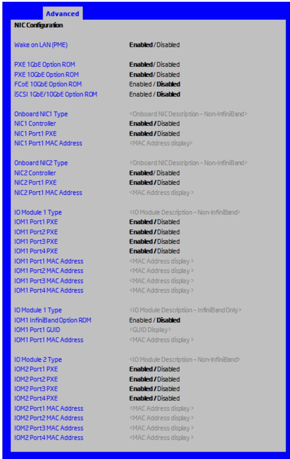
Figure 26. NIC Configuration Screen
