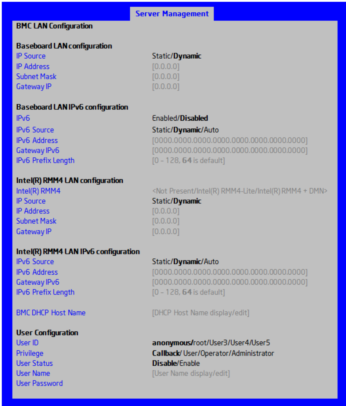
Figure 35. BMC LAN Configuration Screen
