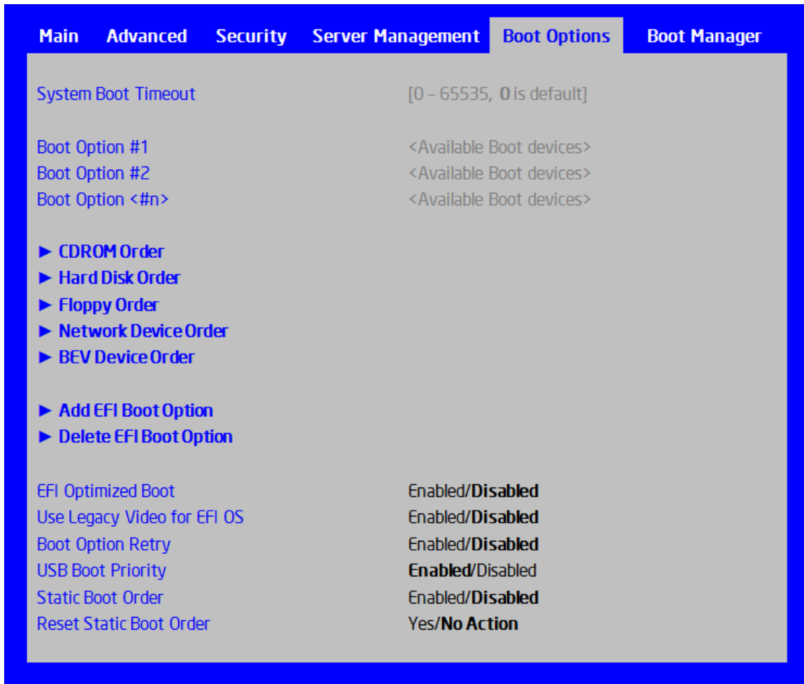
Figure 36. Boot Option Screen
