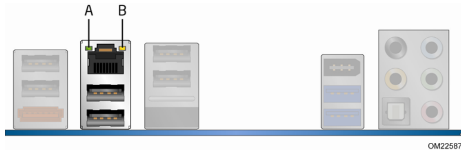
Figure 2. LAN Connector LEDs
